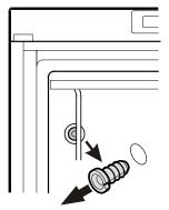
4. Feed sensor through opening and secure sensor cable with
